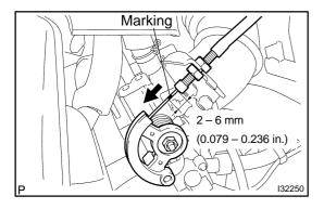
(b) Pull the wire and check the moved distance of the mark.
