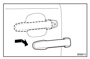
(b) Pushing the outside handle in the arrow mark direction as shown in the illustration, remove the outside handle.
