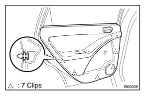
(b) Using a screwdriver, disengage the clips and then pull the trim board upward to remove it.
