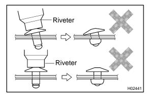
Do not tilt the riveter when removing the rivet, because the materials are not tightened firmly.
