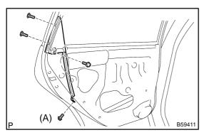
(b) Install the bolt and 3 screws.
