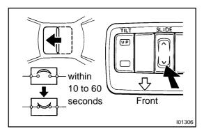
(b) With the sliding roof in the fully opened position, hold the sliding roof switch in the "CLOSE" side and check that the sliding roof begins to close within 60 seconds.
