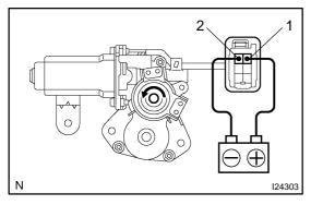
(b) Reverse the polarity, check that the motor turns counterclockwise (moves to the open side).
