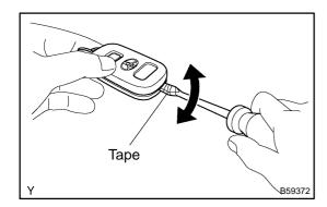
(a) Using a screwdriver, remove the cover.
