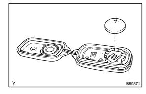
(b) Remove the battery (lithium battery).
