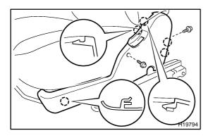
(b) Remove the 2 screws and seat cushion shield inner.
