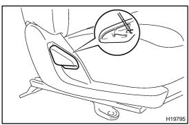
(c) Using a screwdriver, remove the reclining adjuster release handle.
