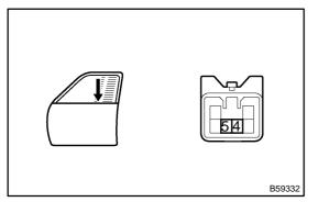
(4) When approximately 60 seconds have elapsed after the inspection of the current cut–off, check that the door glass goes down when the power window regulator switch is turned DOWN.
