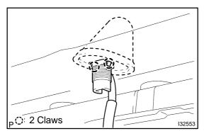
(b) Release the 2 fitting claws, remove the amplifier antenna assy.
