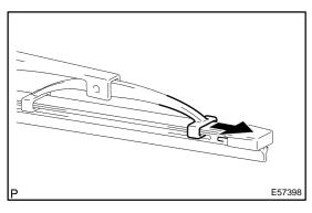
(b) Install the wiper rubber LH so that the head part (Larger side) of the wiper rubber faces the arm axie side.
