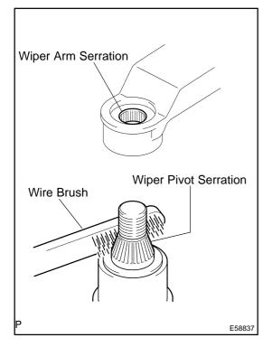
(d) Install the front wiper arm LH with a nut to the position shown in the illustration.
