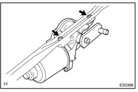
(b) Remove 2 torx bolts and windshield wiper motor assy.
