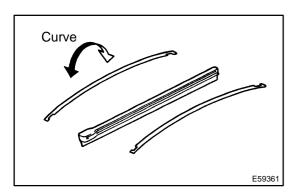
(a) Install the 2 wiper rubber backing plates to the rear wiper rubber.
