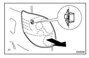
(c) Pull out the rear combination light assy LH to the back of the vehicle, and remove.
