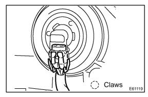
(c) Release the 2 claws and disconnect the connectors as shown in the illustration, and remove the headlight assy LH.
