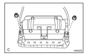
(1) Install the 2 nuts to the instrument panel passenger airbag assy.
