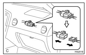
(c) Disconnect the instrument panel passenger airbag connector.
