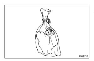
Dispose the instrument panel passenger airbag assy. **CAUTION:**
