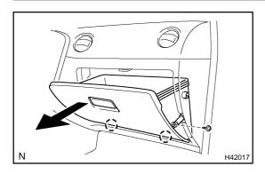
(b) Remove the screw and glove compartment door assy.
