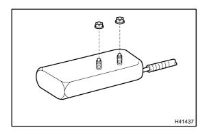
(1) Install the 2 nuts in the front seat airbag assy.
