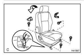
(b) Disconnect the side airbag connector.
