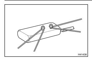
(2) Wind the wire harness around the stud bolts of the front seat airbag assy as shown in the illustration.
