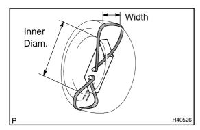
(3) Position the front seat airbag assy inside the tire with the airbag deployment direction facing inside.
