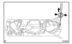
(c) Using a screwdriver, open the claw of the cable clamp and disconnect the airmix damper control cable.
