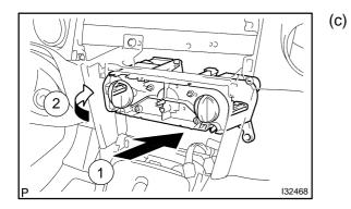
Connect the connector, fit the 2 fitting claws of air conditioning control assy in the instrument panel sub–assy lower hole.
