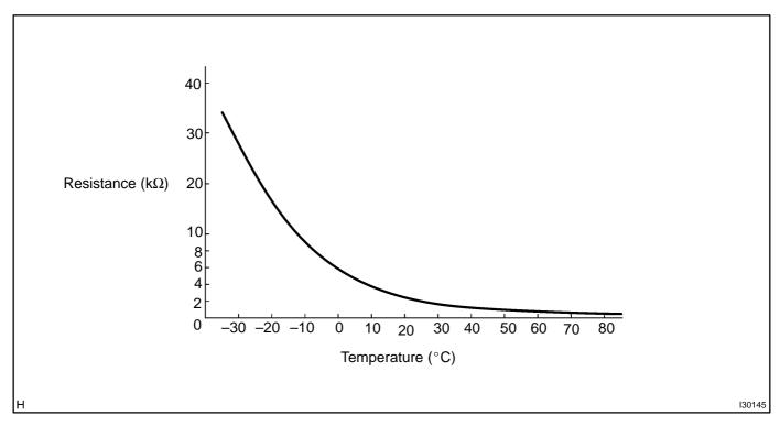
If resistance value is not as specified, replace the sensor.
