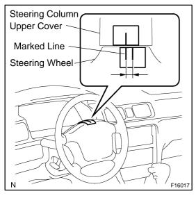
(4) Turn the steering wheel to its straight position.
