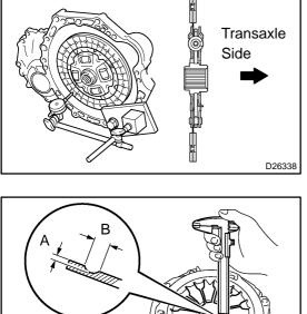
(c) Using a dial indicator, check the clutch disc assy runout. Minimum runout: 0.8 mm (0.031 in.)
