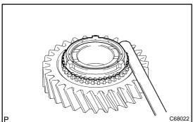
(b) Using a feeler gauge, measure the clearance between the synchronizer ring back and gear spline end.
