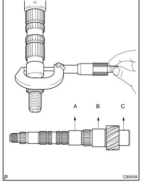
(b) Using a micrometer, measure the outer diameter of the output shaft journal surface.
