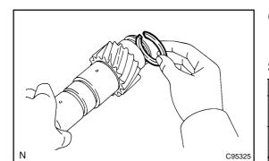
(b) Select a snap ring from the table below that will make the thrust clearance of the output shaft front bearing (inner race) below 0.1 mm (0.004 in.).
