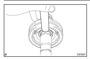
(b) Select a snap ring from the table below that will make the thrust clearance of the transmission clutch hub No.2 below 0.1 mm (0.004 in.).
