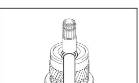
(b) Select a snap ring from the table below that will make the thrust clearance of the input shaft rear radial ball bearing below 0.1 mm (0.004 in.).
