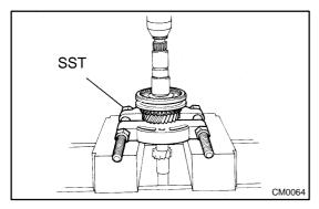
(b) Using SST and a press, remove the transmission clutch hub No.2 and 3rd gear from the input shaft.
