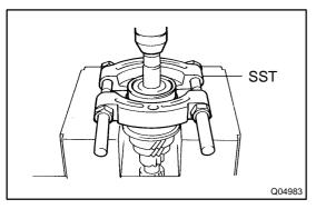
(b) Using SST and a press, remove the input shaft radial ball bearing rear and 4th gear from the input shaft. SST 09950–00020
