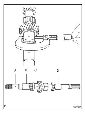
(b) Using a micrometer, measure the outer diameter of the input shaft journal surface.
