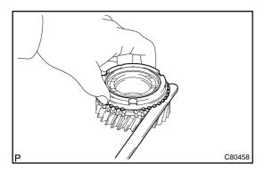
(c) Using a feeler gauge, measure the clearance between 4th gear synchronizer ring back and 4th gear spline end.
