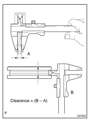
(c) Using a vernier caliper, inspect the transmission hub sleeve No.2 and gear shift fork No.2 as shown in the illustration.
