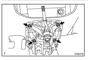
**REMOVE FLOOR SHIFT SHIFT LEVER ASSY** (a) Remove the 4 nuts and shift lever assy.
