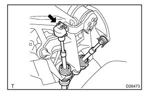
(b) Connect the select cable end with the clip.
