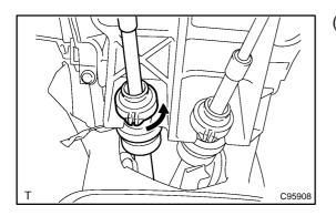
Turn the lock and disconnect the select cable from the (b) shift lever assy.
