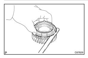
(b) Using a feeler gauge, measure the clearance between the 4th gear synchronizer ring back and 4th gear spline end.
