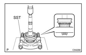
(b) Using SST and a press, remove the transmission clutch hub No.2 with 3rd gear from the input shaft.
