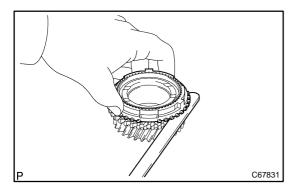
(b) Using a feeler gauge, measure the clearance between the 3rd gear synchronizer ring back and 3rd gear spline end.
