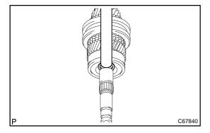
(b) Select a snap ring that will allow minimum axial play.Standard clearance:0.1 mm (0.004 in.) or less
