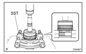
(b) Using SST and a press, remove the input shaft bearing with 4th gear from the input shaft.
