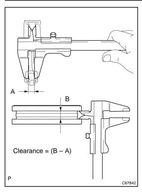
(c) Using a vernier calipers, inspect the transmission hub sleeve No.2 and gear shift fork No.2 as shown in the illustration.
