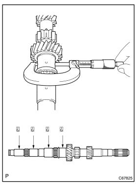
(b) Using a micrometer, measure the outer diameter of the input shaft jurnal surface.
