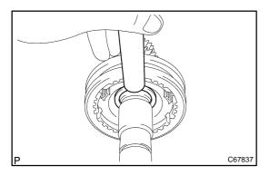
(b) Select a snap ring that will allow minimum axial play.Standard clearance:0.1 mm (0.004 in.) or less
