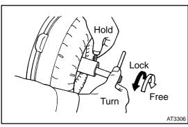
(3) With the torque converter clutch setting up on its side, check that the one-way clutch locks when it is turned counterclockwise, and rotates smoothly clockwise.
