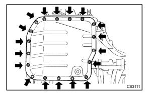
(c) Install a new gasket, oil pan and 18 bolts to the transaxle case.
