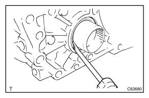
17. **REMOVE FRONT TRANSAXLE CASE OIL SEAL** (a) Using a screwdriver, remove the oil seal.
