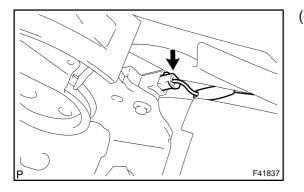
(d) Connect the parking brake switch connector to the parking brake switch.
