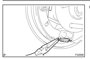
(b) Using a needle–nose pliers, remove the anchor spring.
