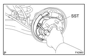
Using SST, remove the 2 cups, shoe hold-down spring and pin, and remove the front brake shoe.
