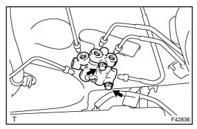
(b) Remove the 2 bolts and proportioning valve assy from the body.
