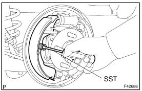
(b) Using SST, install the front brake shoe, pin, shoe hold– down spring and cup.
