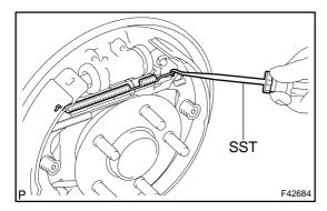
(e) Using SST, install the upper side tension spring with spacer.
