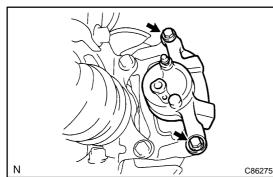
(b) Hold the cylinder slide pin and remove the 2 bolts.
