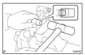
Do not damage the cylinder boot.
