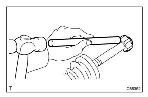
(g) Using a brass bar and a hammer, remove the inner race. **NOTICE:**
