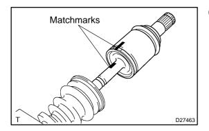
(g) Align the matchmarks, install the inboard joint assy LH to the outboard joint shaft assy LH.
