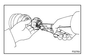
(f) Using a snap ring expander, remove the rear drive shaft LH snap ring.
