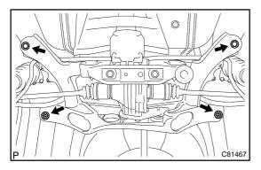
(b) Remove the 2 bolts and 2 nuts from the rear suspension member sub–assy.
