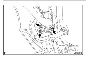
(c) Remove the front side 3 bolts and rear suspension arm assy No.1 LH.
