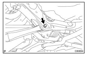
(b) Remove the bolt and nut, disconnect the rear side rear suspension arm assy No.1 LH.
