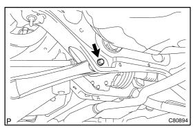
(f) Remove the bolt and nut, separate the rear side rear suspension arm assy No.1 LH.
