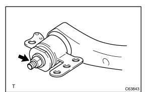
(h) Remove the nut, rear suspension arm bracket assy LH and rear suspension support stopper.
