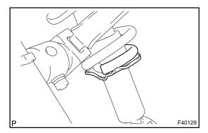
(b) Insert the coil spring rear LH into the shock absorber assy rear LH.
