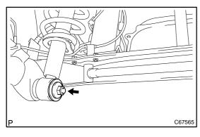
(b) Install the rear shock absorber with coil spring, temporarily tighten the nut and rear shock absorber LH cushion retainer.
