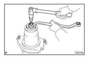
(j) Use a 6 mm hexagon wrench to hold the piston rod and tighten the nut.
