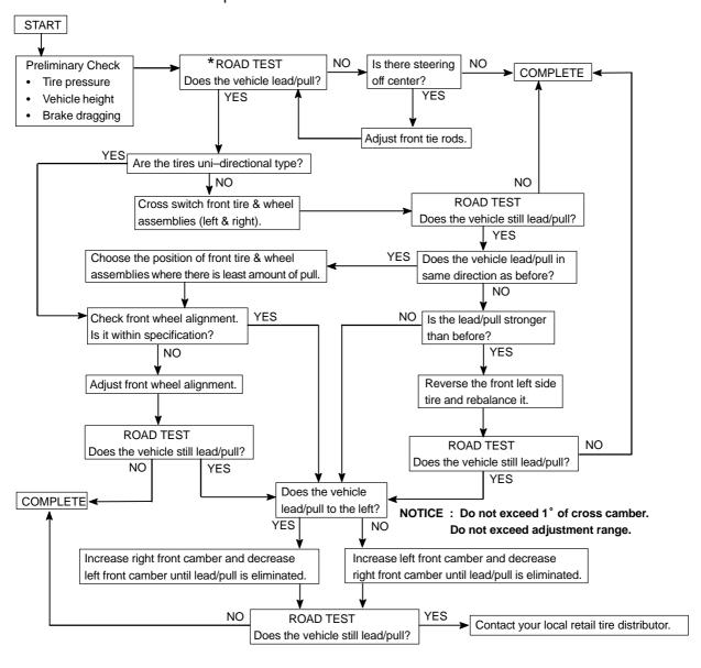
Select a flat road where the vehicle can be driven in a straight line for 100 meters at a constant speed of 35mph. Please confirm safety and set the steering wheel to its straight position. Drive the vehicle in a straight line for 100 meters at a constant speed of 35 mph without holding the steering wheel.
