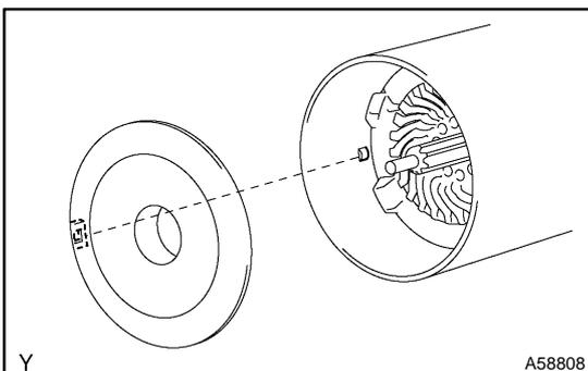
**12. INSTALL STARTER ARMATURE PLATE**
