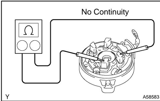
**8. INSPECT STARTER COMMUTATOR END FRAME ASSY**
