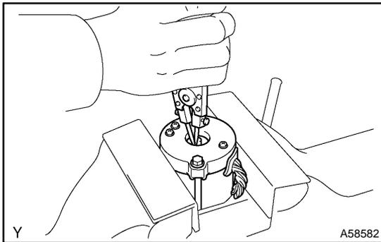
**3. REMOVE STARTER COMMUTATOR END FRAME ASSY**
