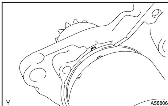
**16. INSTALL STARTER COMMUTATOR END FRAME ASSY**
