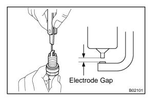
(c) Check the spark plug electrode gap.
