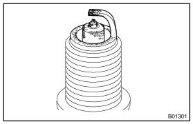
(b) Check the spark plug for thread damage and insulator damage.
