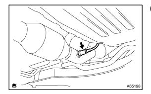
(c) Remove the oxygen sensor.
