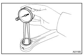
(c) Using a caliper gauge, measure the connecting rod small end bore diameter.
