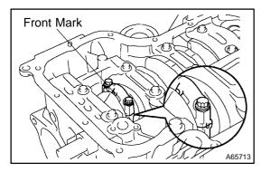
(e) Align the pin dowels of the connecting rod cap with the pins of the connecting rod, and install the connecting rod.
