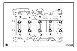
(j) Uniformly loosen the 10 bearing cap bolts, in several passes, in the sequence shown in the illustration.
