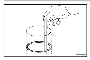
(b) Using a feeler gauge, measure the end gap.
