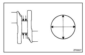
(b) Using a micrometer, measure the diameter of each main journal at the points shown in the illustration.
