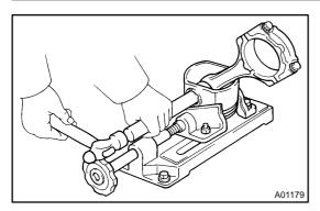
(c) Using a plastic hammer and brass bar, lightly tap out the piston pin and remove the connecting rod.
