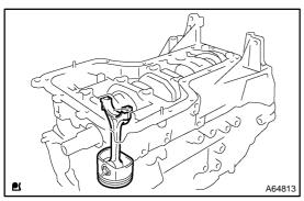
(b) Push the piston, connecting rod assembly and upper bearing through the top of the cylinder block.
