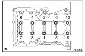
(e) Using SST, tighten the bolts in several passes, in the sequence shown, by the specified torque.
