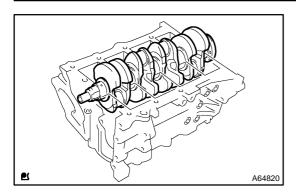
(d) Remove the crankshaft from the cylinder block.
