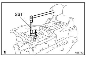
(I) Remove the 2 bolts and connecting rod cap.
