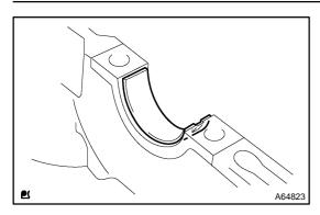
(b) Remove the 5 crankshaft bearings from the bearing cap. **NOTICE:**
