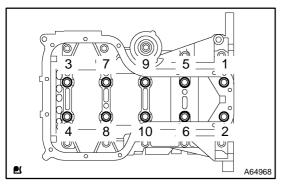
(b) Uniformly loosen the 10 bearing cap bolts, in several passes, in the sequence shown in the illustration. SST 09011–38121
