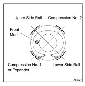
(c) Position the piston rings so that the ring ends are as shown.
