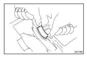
(b) Install the lower bearing on the bearing cap sub–assy. **NOTICE:**
