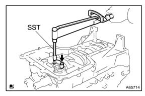
(h) Using SST, tighten the bolts in several passes by the specified torque.
