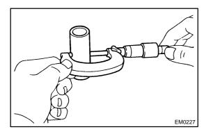
(b) Using a micrometer, measure the piston pin outer diameter.
