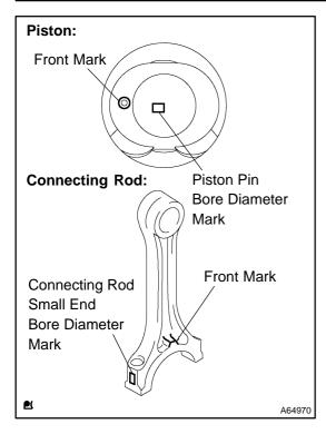
(d) Subtract the piston pin outer diameter measurement from the piston pin bore diameter measurement.
