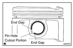
(d) Using a small screwdriver, install a new snap ring at one end of the piston pin hole.
