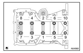
(d) Using SST, tighten the bolts in several passes, in the sequence shown, by the specified torque.
