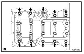
(h) Tighten 10 other bolts for the bearing cap.
