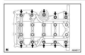
(i) Tighten 10 other bolts for the bearing cap.
