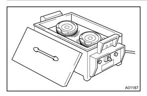
(b) Heat the piston to  $80 - 90^{\circ}\text{C}$  (176–194°F).
