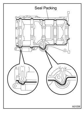
(d) Apply seal packing in the shape of bead (Diameter 2.5 – 3.5 mm (0.098 – 0.139 in.) consequently as shown in the illustration.
