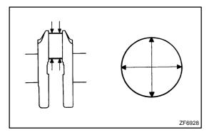
(d) Using a micrometer, measure the diameter of each crank pin at the points shown in the illustration.
