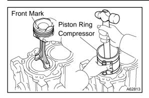
(d) Using a piston ring compressor, push the correctly numbered piston and connecting rod assemblies into each cylinder with the front mark of the piston facing forward.
