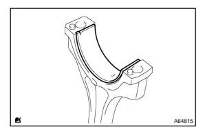
(b) Remove the connecting rod bearing from the connecting rod.
