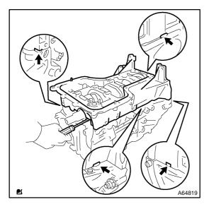
(c) Using a screwdriver, remove the bearing cap by prying the indicated portions between the cylinder block and bearing cap.
