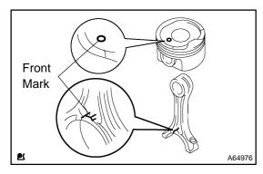
(c) Align the front marks on the piston with connecting rod, and push in the piston with your thumb.
