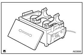
(b) Heat the piston to  $80 - 90^{\circ}\text{C}$  (176 - 194°F).
