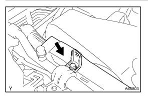
6. INSTALL WIRE HARNESS CLAMP Torque: 10 N·m (102 kgf·cm, 7 ft·lbf)
