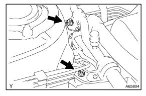
5. INSTALL SUCTION HOSE SUB-ASSY Torque: 9.8 N·m (100 kgf·cm, 87 in.·lbf)
