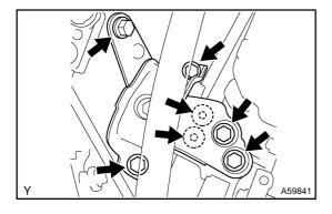
(b) Remove the 5 bolts, 2 nuts and engine mounting insulator sub–assy RH.
