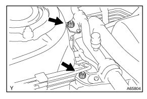
16. INSTALL SUCTION HOSE SUB-ASSY Torque: 9.8 N·m (100 kgf·cm, 87 in.·lbf)
