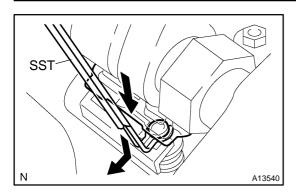
(c) Lift the rocker arm to make a room and use SST, install the adjusting shim.
