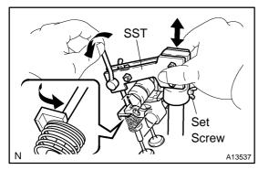
(3) Operate the lever so that SST's seat surface comes to contact with the valve retainer and lock them with the set screw.
