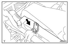
17. INSTALL WIRE HARNESS CLAMP Torque: 10 N·m (102 kgf·cm, 7 ft·lbf)
