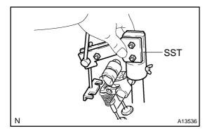
(2) Insert SST into the plug tube. SST 09248–77010 (09248–07010)
