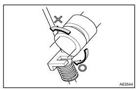
(d) Turn the crankshaft so that the related rocker arm, where the valve clearance is adjusted, is fully pushed down.
