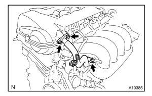
(g) Install a new gasket and No. 1 ventilation pipe with 2 nuts and bolt.
