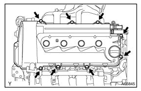
(e) Install the cylinder head cover and wire harness protector with the 8 bolts. Uniformly tighten the bolts, in the several passes, in the sequence shown.
