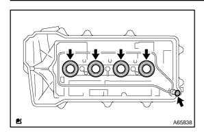
(d) Install the new spark plug tube gasket and a new O-ring to the cylinder head cover.
