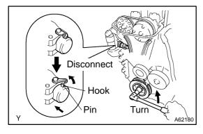
(3) Turn the crankshaft counterclockwise, and disconnect the plunger knock pin from the hook.
