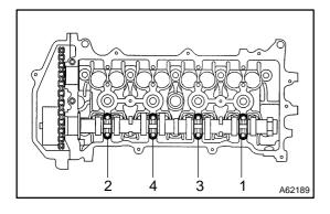
(g) Loosen the camshaft bearing cap bolts on camshaft in the order as shown in the illustration in several passes, and remove the caps.
