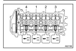
(n) Examine the front marks and numbers and tighten the bolts in the order shown in the illustration.
