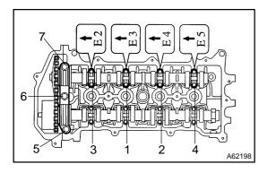
(q) Examine the front marks and numbers and tighten the bolts in the order shown in the illustration.
