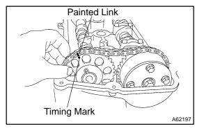
(o) Put the camshaft No.2 on the cylinder head with the painted links of the chain aligned with the timing mark on the camshaft timing sprocket.
