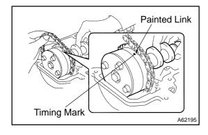
(m) As shown in the illustration, install the timing chain on the camshaft timing gear, with the painted links aligned with the timing marks on the camshaft timing sprocket.
