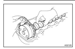
(h) Remove the camshaft with holding the timing chain.
