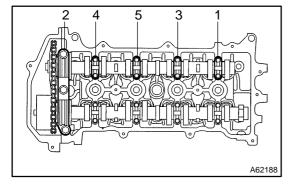
(e) Loosen the camshaft bearing cap bolts on No. 2 camshaft in the order as shown in the illustration in several passes, and remove the caps.
