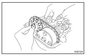
(p) Tighten the camshaft timing gear set bolt temporarily.
