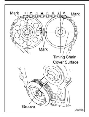
(t) Check the match marks on the timing chain and camshaft timing sprockets, and then the alignment of the pulley groove with timing mark of the chain cover as shown in the illustration.
