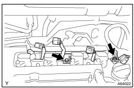
(c) Remove the bolt and nut installing the engine wire.
