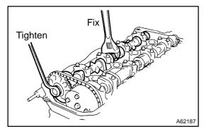
(s) Fix the camshaft with a spanner and so on, then tighten the camshaft timing gear set bolt.
