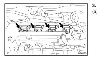
(a) Remove the 4 bolts and 4 ignition coils.
