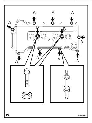
(c) Install the cylinder head cover and cable bracket with the 9 bolts, 2 seal washers and 2 nuts. Uniformly tighten the bolts and nuts, in the several passes.
