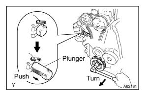
(4) Turn the crankshaft clockwise, and check that the slipper is pushed by the plunger.
