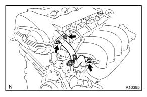
(g) Install a new gasket and No. 1 ventilation pipe with 2 nuts and bolt.
