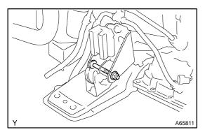
(c) Install the bolt holding the front engine mounting bracket to the mounting insulator. Torque: 52 N·m (530 kgf·cm, 38 ft·lbf)
