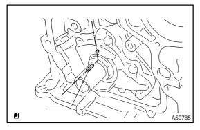
(2) Turn the crankshaft and set the set key on the crankshaft upward.
