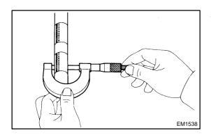
51. INSPECT VALVE ROCKER SHAFT SUB-ASSY NO.2
