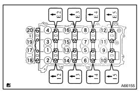
(c) Examine the front marks and numbers and tighten the bolts in the order shown in the illustration.
