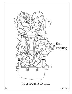
(e) Install the timing chain cover, with the 13 bolts. **Torque:**
