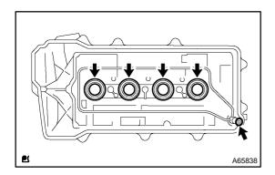
(c) Install the new spark plug tube gasket and a new O-ring to the cylinder head cover.
