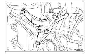
9. REMOVE TRANSVERSE ENGINE ENGINE MOUNTING BRACKET
