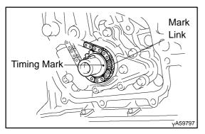
(b) Install the timing chain on the crankshaft timing sprocket with the mark link (yellow color link) aligned with the timing mark on the crankshaft timing sprocket.
