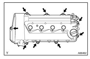
(e) Install the cylinder head cover and cable bracket with the 9 bolts.
