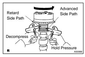
(4) Confirm if the camshaft timing gear assembly revolves in the timing advance direction when weakening the air pressure of the timing retard path.
