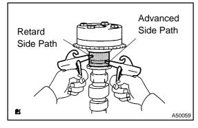
(3) Put air pressure into two broken paths (the advance side path and the retard side path) with about 150 kPa {1.5 kgf/cm²}.
