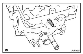
(b) Remove the oil control valve filter.(Rear side)
