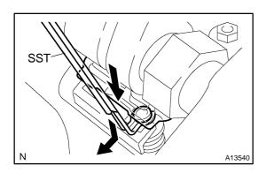
(c) Lift the rocker arm to make a room and use SST, install the adjusting shim.
