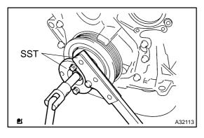
(b) Using SST, remove the pulley bolt. SST 09213-70011 (09213-70020), 09330-00021
