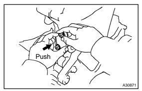
(b) Apply engine oil to the chain tensioner and install it. **Torque: 9.0 N·m (92 kgf·cm, 80 in.·lbf)**
