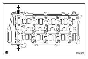
(d) Apply seal packing to 2 locations as shown in the illustration.
