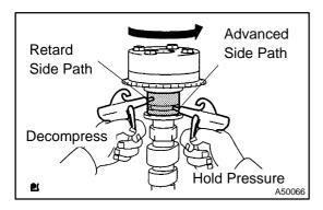
(e) Confirm if the camshaft timing gear assembly revolves in the timing advance direction when weakening the air pressure of the timing retard path.
