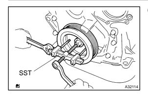
(c) Using SST, remove the crankshaft pulley. SST 09950–50013 (09951–05010, 09952–05010, 09953–05020, 09954–05021)
