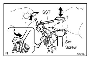
(2) Operate the lever so that SST's seat surface comes to contact with the valve retainer and lock them with the set screw.
