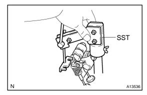
(1) Insert SST into the plug tube. SST 09248–77010(09248–07010)
