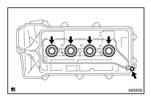
(b) Remove the spark plug tube gasket and O-ring.
