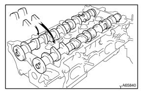
(b) Place the 2 camshafts on the cylinder head with the No.1 cam lobes facing as shown the illustration.
