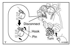
(c) Turn the crankshaft counterclockwise, and disconnect the plunger knock pin from the hook.
