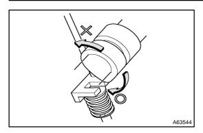
(d) Turn the crankshaft so that the related rocker arm, where the valve clearance is adjusted, is fully pushed down.
