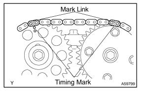
(d) Install the timing chain on the camshaft timing sprockets with the mark link (orange color links) aligned with the timing marks on the camshaft timing sprockets.
