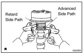
(d) Put air pressure into two broken paths (the advance side path and the retard side path) with about 150 kPa {1.5 kgf/ cm<sup>2</sup>}.
