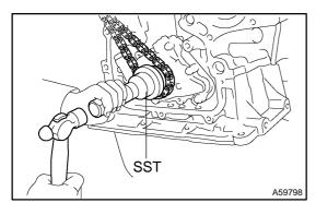
(c) Using a SST, install the sprocket. SST 09223–22010
