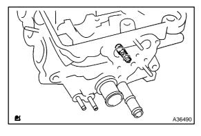
(c) Install the oil control valve filter from the cylinder head.(Rear side)
