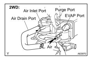
(3) While holding the purge port and the air drain port closed, blow air (1.76 kPa, 18 gf/cm², 0.26 psi) into the EVAP port and check that air does not flow from the air inlet port.
