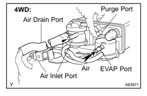
(4) Apply vaccum (3.43 kPa, 25.7 mmHg, 1.01 in.Hg) to the purge port, check that the vacuum dose not decrease when the air inlet port is closed, and check that the vacuum decreases when the air inlet port is released.
