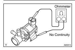
(2) Using an ohmmeter, check that there is no continuity between each terminal and the body.
