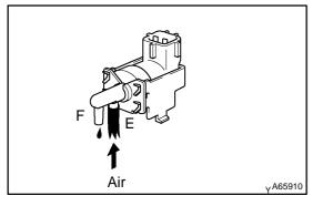
(3) Check that air does not flow from ports E to F.
