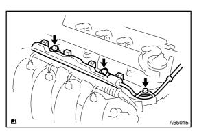
(c) Remove the 3 bolts and fuel delivery pipe together with the 4 fuel injectors and fuel tube.
