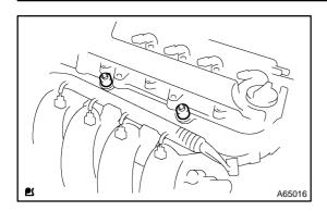
(d) Remove the 2 spacers from the cylinder head.
