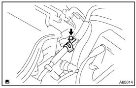
(b) Remove the bolt and clamp.
