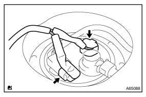
(b) Disconnect the fuel pump and vapor pressure sensor connector.
