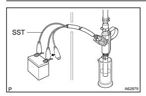
(5) Put the fuel injector into a graduated cylinder.
