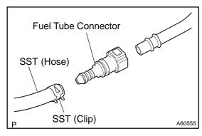
(2) Connect SST and fuel tube connector to the fuel pipe.
