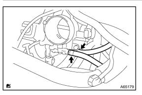
(d) Disconnect 2 water by–pass hoses from the throttle body.
