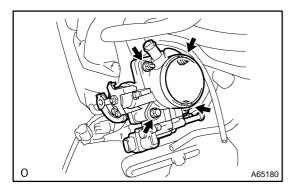
(e) Remove the throttle body and accelerator control cable bracket with 2 bolts and 2 nuts.
